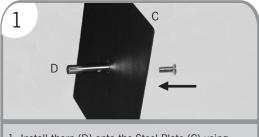
1. Install thorn (D) onto the Steel Plate (C) using the screw.
